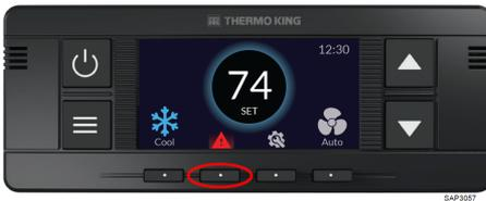
The Alarms list will appear displaying all active Shutdown (Red), Check (Amber), and Log (Yellow) alarms. The HMI Alarm screen displays up to 32 active alarms in priority order to assist in troubleshooting. Select an alarm for specific details. The option to Clear an alarm may or may not be available depending on the alarm type.
